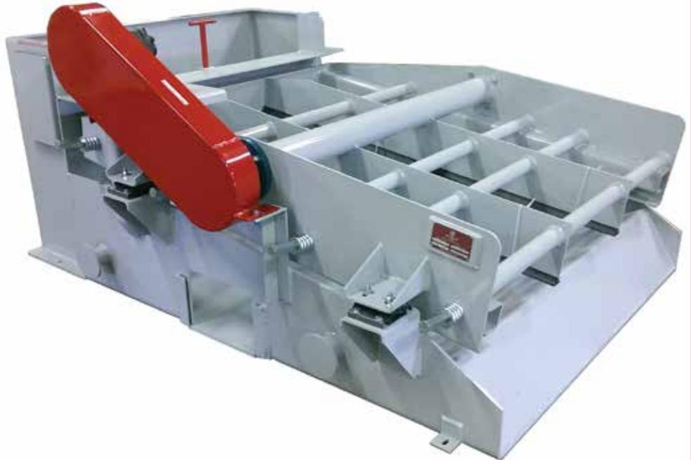
**DLC 4X5 SINGLE STANDARD** Shale Shaker has been designed to provide extended service life in all drilling related applications for which it was designed. Each unit is constructed of A-36 and/or 316ss plate built to proven oilfield specifications. The vibrating assembly can be powered by an electric motor or a hydraulic motor.
